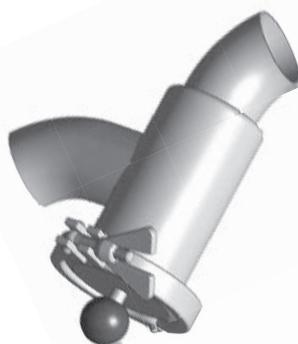
AWH dirt traps protect your product and plant components, pumps, heat exchangers etc., from foreign objects that can cause malfunctions. Our dirt traps are Y-shaped (Y filter). The direction of flow is always from the inside to the outside. The trap should be installed so that the filter insert is removed from below. Its streamlined shape ensures reliable processes in a simple and cost-effective way.
