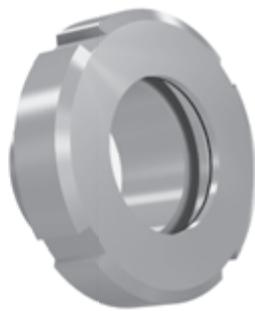
1. In the standard sight glass, a pane of tempered glass is screwed in to a male with a welded end using a seal ring and a grooved nut. The sight glass is made of Borosilicate glass, which offers excellent strength and thermal stability. The maximum temperature is 280 °C (acc. to DIN 7080). The change in temperature from 230 °C to 20 °C must take at least 1 minute.
